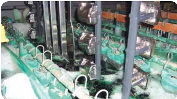
*In Elite/RPW’s process,, the nickel solution (foamy liquid above) is recycled. The spray-off system is also part of Elite/RPW’s recovery system.*
